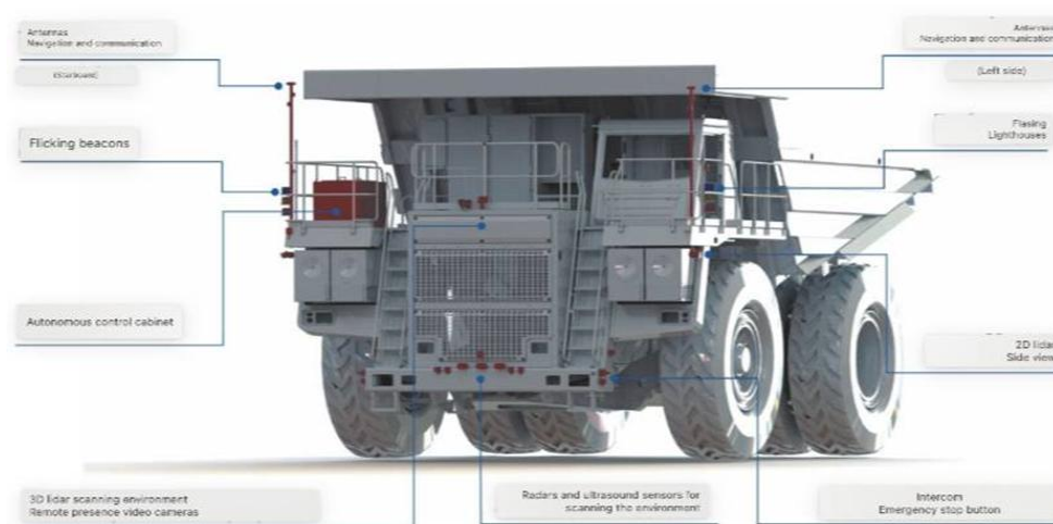
Fig. 2. BELAZ 7513 series dump truck with on-board equipment of a robotic mobile system
