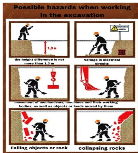
Figure 2. Possible hazards when working in the excavation
